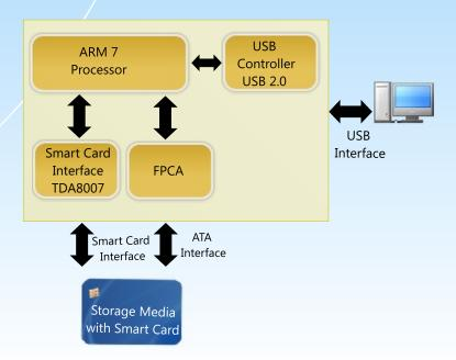
It is a USB composite device with two different interfaces mass storage and CCID. The reader authenticates the user before providing access to data stored on the storage media. This device supports AES based data encryption and PKI authentication.
